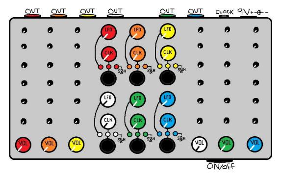
Each control circuit is simply powering a 40106 which then provides all the oscillators. An analog LFO is run into a LF398 chip that is being clocked by a microcontroller which lets us control the 40106 in three different modes:
